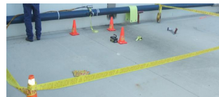
Figure 2: 10' x 10' restricted area using a SCAR exposure device
