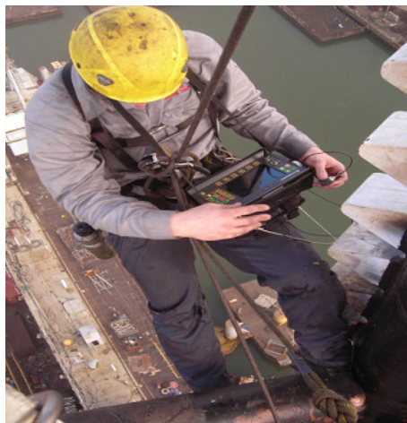
Figure 2: Manual Ultrasonic Shear Wave (UTSW) testing
