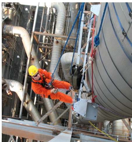
Figure 1: Imager real-time radiography (RTR)
