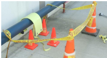
Figure 3: 4' x 4' restricted area using a SCAR exposure device with additional shielding
